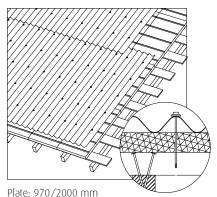
Roof Ridge; 48.5x2000 mm Veneer Board 2/12 Monoblock nail with galvanized plastic cap; 10 cm. EPS or XPS
