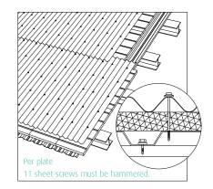
Plate; 970/2000 mm Roof Ridge; 48.5x2000 mm EPS or XPS 065mm trapezoidal sheet 27/200 6. 3x22 drill-point screw 20 nails must be hammered. Drill-tipped screw Steel purlin
